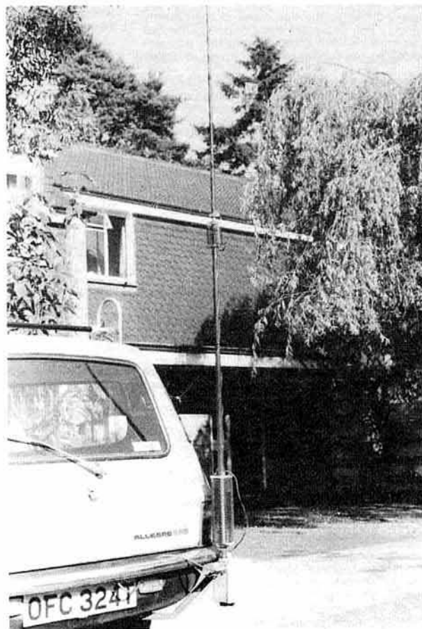
Photo 1. The whip antenna mounted with both centre and base loading coils. The base coil is shown completely bypassed. The two twisted copper strips are clearly seen on the bottom section
