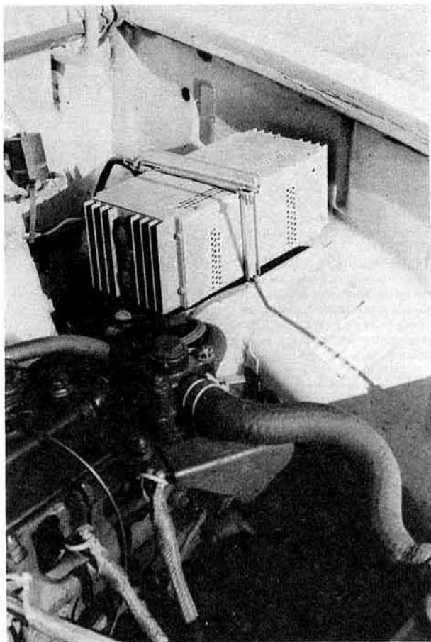
Photo 4. Another view showing a little more clearly the connections between the braid and the cans screening the plugs. The mounting arrangements for the power supply are also clearly illustrated
